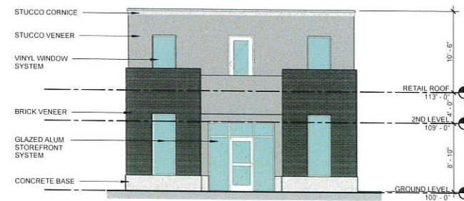
01 NW BUILDING - WEST ELEVATION 1/8" = 1'-0"
