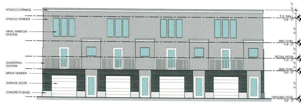
03 SW BUILDING - EAST ELEVATION 1/8" = 1'-0"
