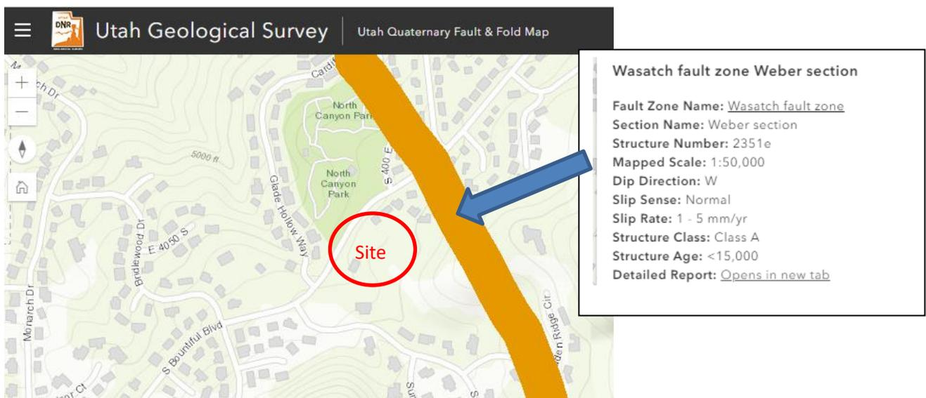
Any future owner of Lot 2 should expect to encounter differing soil conditions on the site and the potential for adverse effects from a seismic event, based on the site’s proximity to the Weber section of the Wasatch fault.
