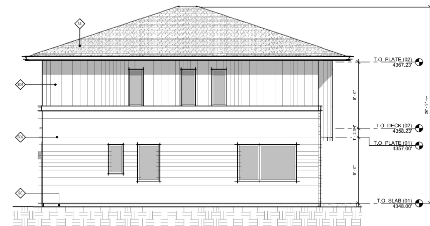
SOUTH (SIDE) ELEVATION A3 1/4" = 1'-0" X/E2010
