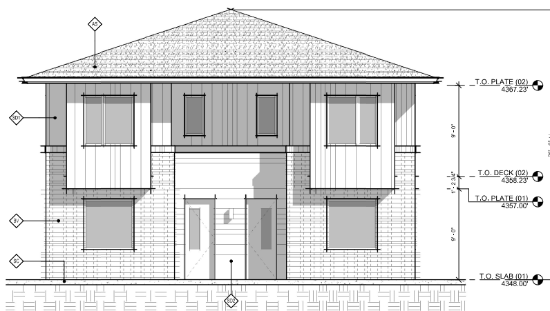
EAST (COURTYARD) ELEVATION (A5) 1/4" = 1'-0" X/E2010
