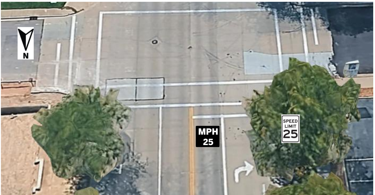
Figure 2 Proposed pavement message and speed limit sign installation at 200 N
