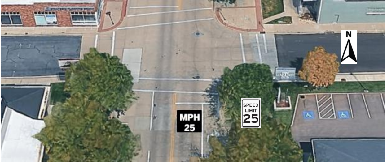
Figure 1 Proposed pavement message and speed limit sign installation at 200 S
