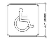
PAINTED EMBLEM ON ASPHALT PAVING TYP. AT ALL ADA PARKING STALLS PER CITY REQUIREMENTS. (2 COATS)
