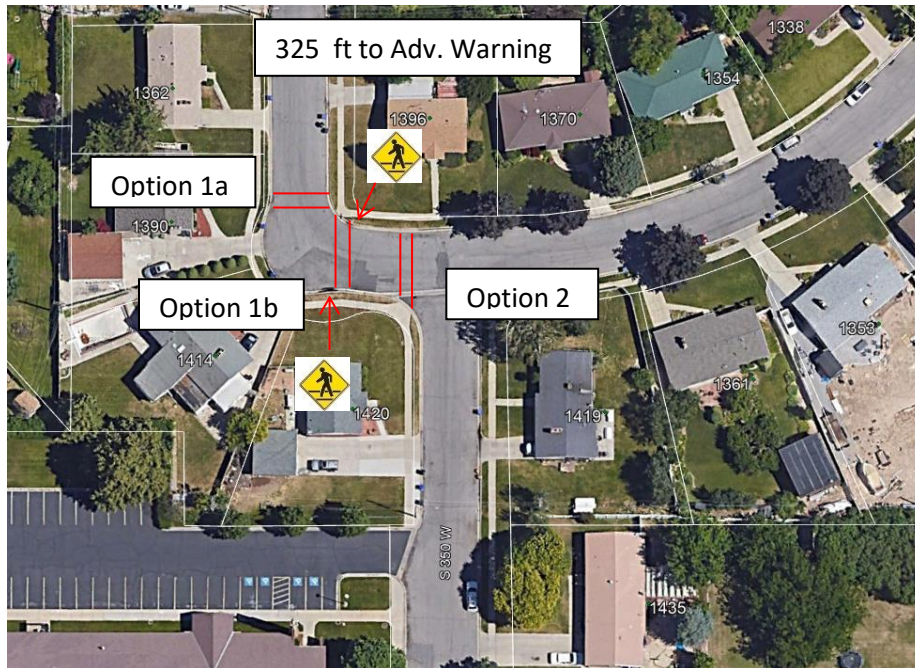
Figure 1 350 W / 1400 S intersection with proposed crosswalk configuration.
