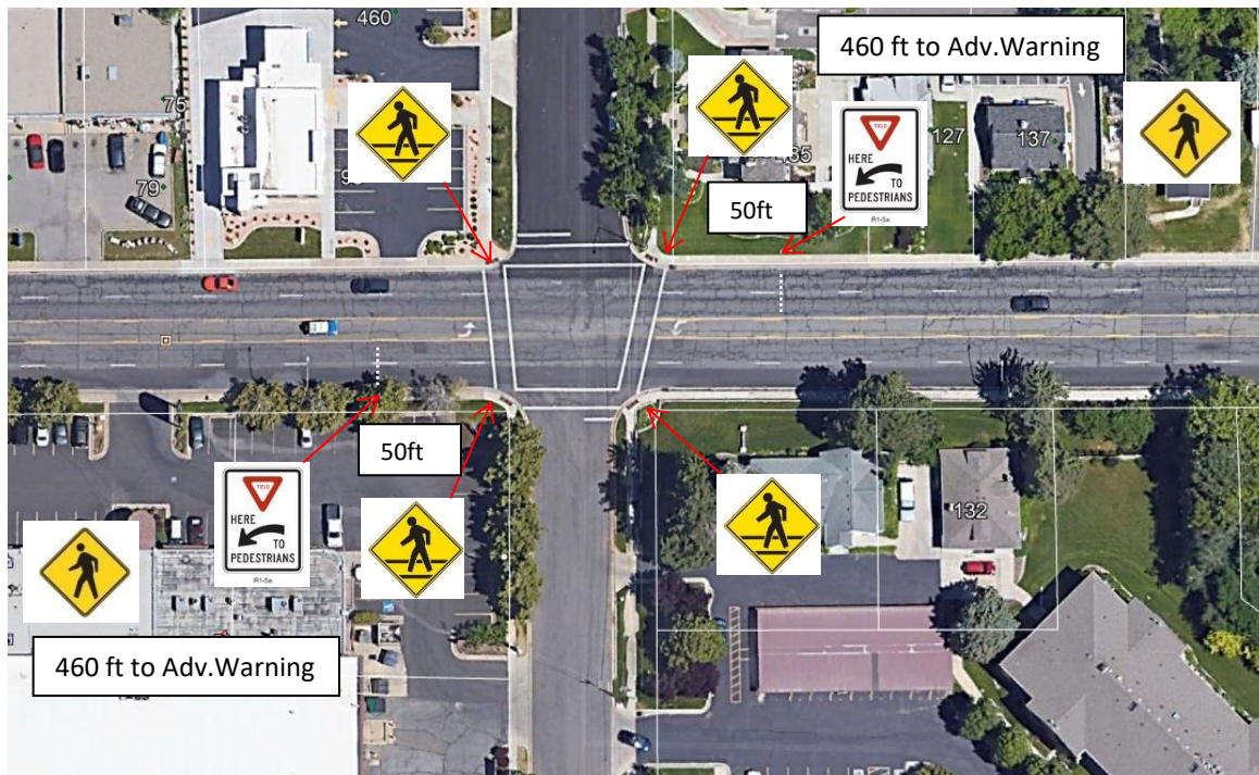
Figure 2 Proposed Improvements at 500 S 100 E Intersection
