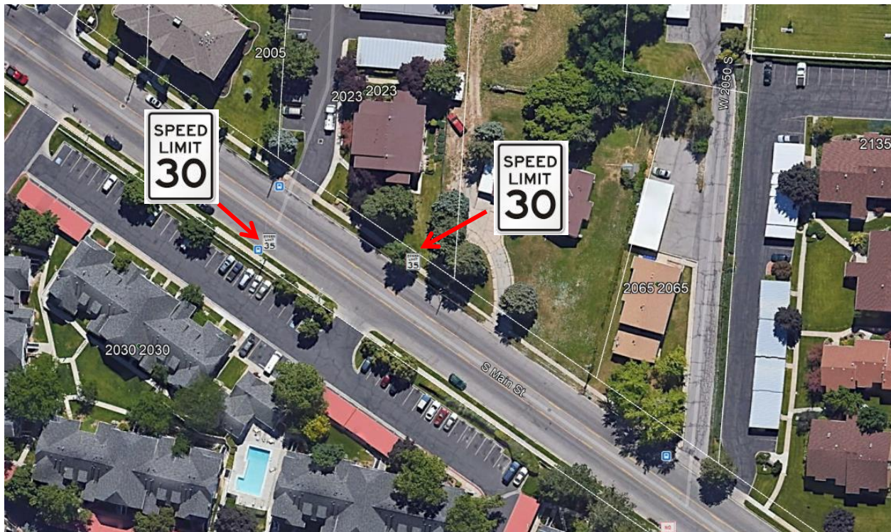
Figure 3 Replace existing 35 mph signs with 30 mph signs
