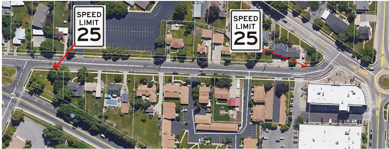
Figure 1 Suggested locations for speed limit signs
