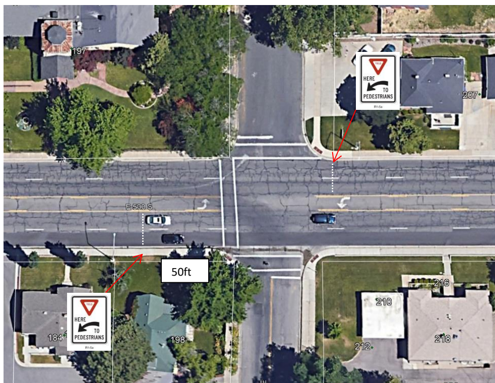
Figure 3 Proposed improvements at the 200 E intersection
