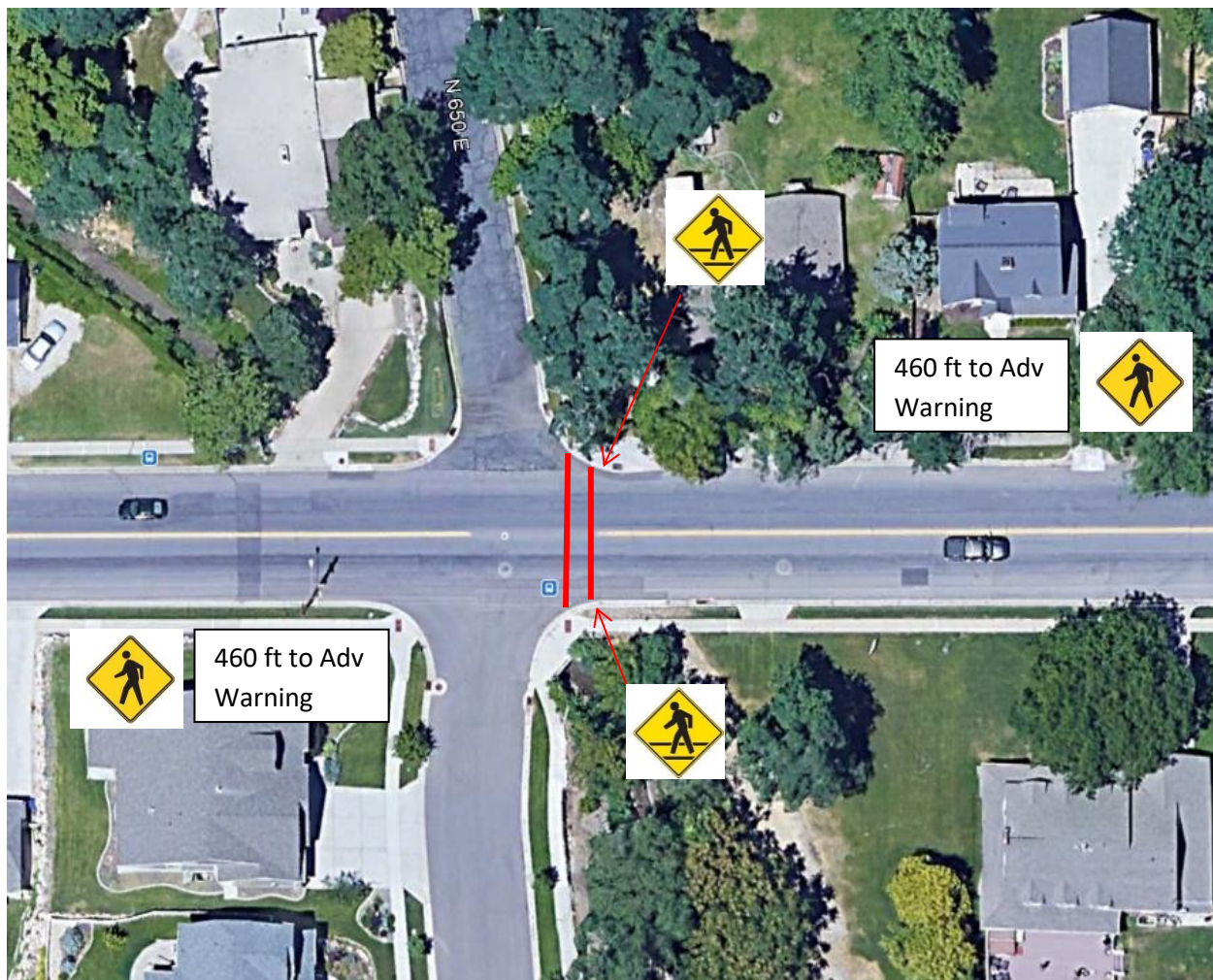
Figure 1 650 E / 400 N intersection with proposed crosswalk configuration.
