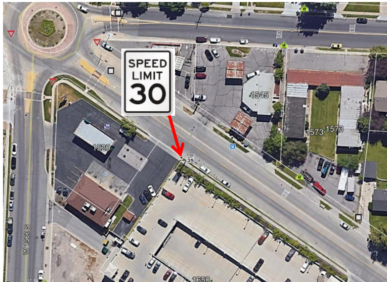
Figure 1 Replace existing 35 mph sign with 30 mph sign
